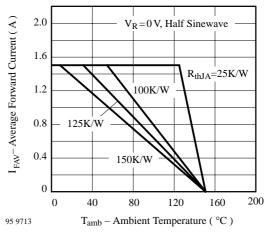
Figure 4. Max. Average Forward Current vs. Ambient Temperature
