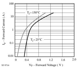
Figure 5. Max. Forward Current vs. Forward Voltage
